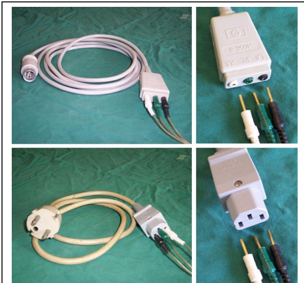
Fig. 1: Murphy's Law illustrated. 2mm male pins of old-style ECG-electrode lead wires normally plug into an ECG patient cable (both upper photos). These pins also fit into worldwide used female IEC mains plug (both lower photos).
